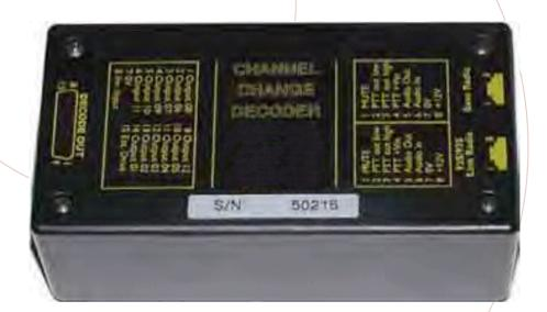
ual Tone Multiple Frequency, (DTMF), is a popular and reliable signalling method used for channel change and other simple control functions. BISS Tech has developed the 970DD as a "building block" to provide an easy interface for equipment requiring DTMF control. The 970DD has been specifically designed to easily interface with the BISS Tech 900 series of radio control modules, but is flexible enough to be used as a stand alone unit for custom projects.
